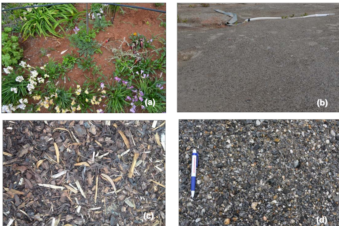
Figure 2. Examples of the main abatement materials used in Broken Hill; (a) garden loam, (b) cracker dust, (c) wood chips and (d) blue metal/road base.
