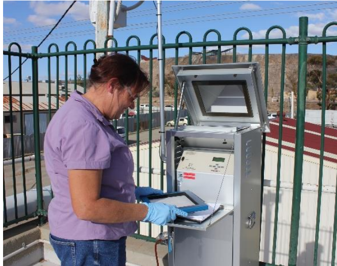
Technical officer, Frances Boreland changes an air filter on a high-volume air gauge
