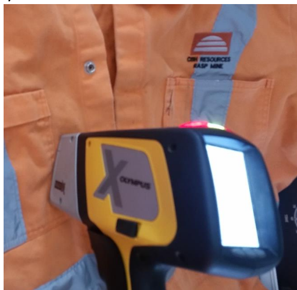
A portable X-Ray fluorescence machine measures the amount of lead in a mine worker's washed clothing.
