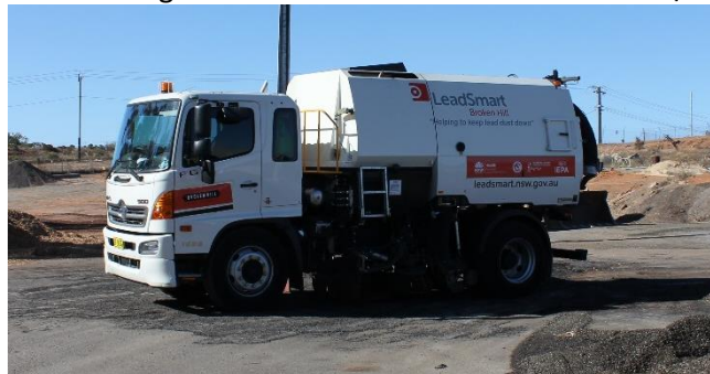
A BHCC street sweeper fitted was fitted with an extra dust control microspray system.
